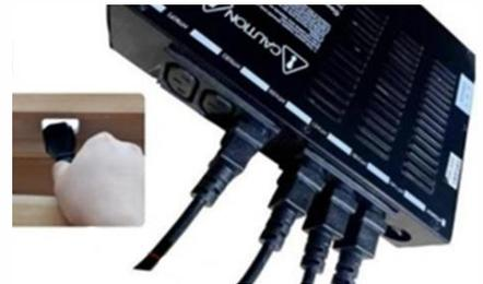
3. Connect the power cables between the control unit and the stove.
